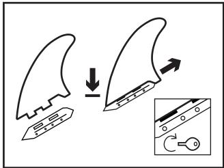
3. Attach fins to fin box, push back to secure. Gently tighten grub screws with fin key (do not overtighten)
