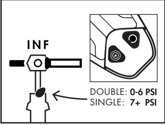
2. Connect hose to INF connection on pump. Use double action setting on pump for first inflation stage, then flip switch to single for higher pressure inflation. Recommended 12-14 PSI max
