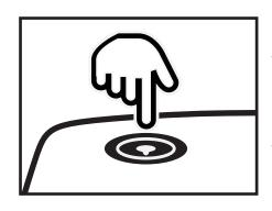
1. Unscrew valve cap, press down to open valve
