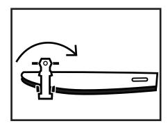
5. Place pump at nose, roll board around pump
